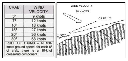
RELATIONSHIP OF CRAB ANGLE AND WIND VELOCITY Air Speed, 100 Knots - Wind Perpendicular to Ridge
