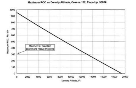
© 1996 Flight Physics, Billings, Montana FIGURE 7 - MAXIMUM RATE OF CLIMB v. DENSITY ALTITUDE, CESSNA 182
