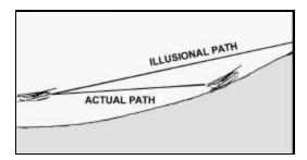
Pulling up to avoid the terrain often causes a stall due to slow airspeed.  $\checkmark$  Never fly perpendicular toward rising terrain.  $\checkmark$  Approach at a 45-degree angle or circle before continuing.
