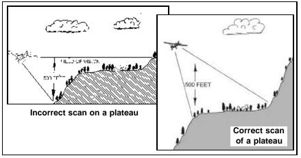
The proper scan while searching a steep slope is illustrated here. Descending 500 feet at the completion of each circuit works well as long as the slope is steep.
