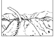
The aircraft is approaching a ridge at a 45-degree angle. A downdraft is present, but the airplane has to get close to the ridge before experiencing its effect.
