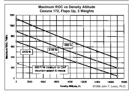
FIGURE 1 - Maximum ROC vs. Density Altitude
