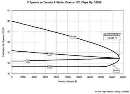
FIGURE 8 - V SPEEDS v. DENSITY ALTITUDE - CESSNA 182
